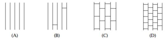
**29** Four polymer samples were tested in a laboratory. Which sample is made from an elastomer?
